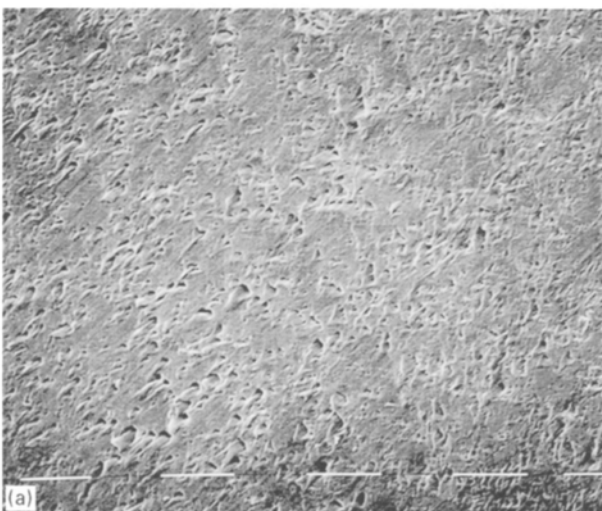
Figure 2 (a) SEM micrograph of PHBVPCL 91 M smoothed surface before etching (1250 \times ), marker size = 10 \mu\text{m} ; (b) SEM micrograph of PHBVPCL 91 M smoothed surface after 5 min THF etching (1250 \times ), marker size = 10 \mu\text{m} .
